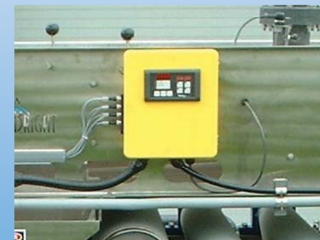
ON PRESS OPERATOR CONTROL STATION
